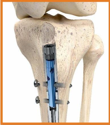
**Figure 1:** *Micromotion locking with the Apex Tibial Nailing System allows 1 mm of controlled cyclic axial compression during weightbearing by means of a preassembled proximal stem insert.*
