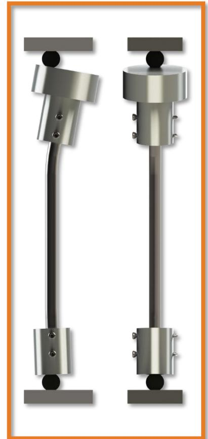
**Figure 2:** *Samples were presented in the fatigue test fixture using composite tubes and ball mounts.*
